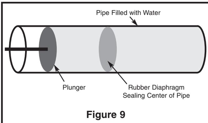
If the pipe had a plunger on one end, as shown in Figure 9, and the plunger was pushed toward the diaphragm, the water in the pipe would force the rubber to stretch out until the force of the rubber pushing back on the water was equal to the force of the plunger. You could say the pipe is charged and ready to push the plunger back. In fact, if the plunger is released it will move back to its original position. The pipe will then be discharged or with no charge on the diaphragm.
